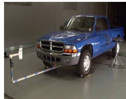
Figure 4 - On road wind velocity measurement using boom anemometer
