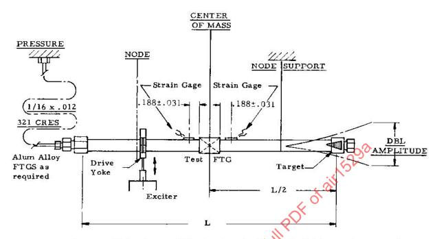
NOTE: In order to eliminate possible damping by the coiled tube, a hose may be connected to a valve at the end of the specimen. After pressurizing, the hose may then be disconnected. However, the mass of the valve must be balanced by an equivalent mass at the opposite end of the specimen. The total increased mass will affect the amplitude. Therefore new tube lengths must be calculated.
