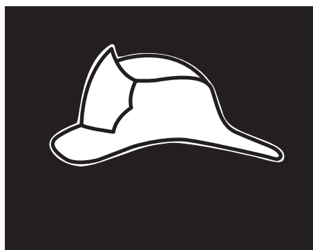
FIGURE 54.12.9 Fire Service Access Elevator Symbol.
