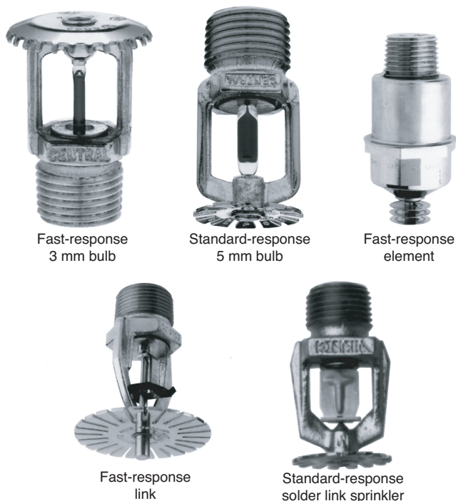
FIGURE A.5.3.1.1 Sprinkler Operating Element Identification.
