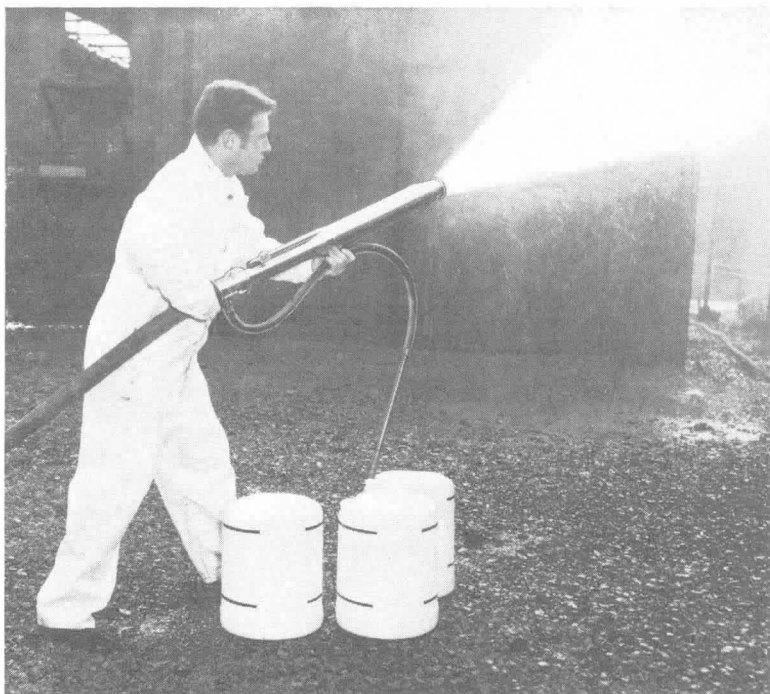
Fig. A-121(a). Air foam nozzle with built-in inductor.
