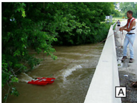
Figure 2 — Photographs showing acoustic Doppler profilers deployed on a small, tethered boat (A) and a power boat (B)
