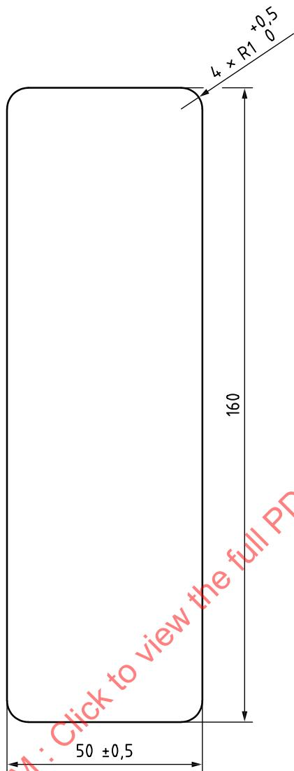
All radii marked shall be 1,0 mm with a tolerance of 0 mm to +0,5 mm. The horizontal dimension shall be 50 mm ± 0,5 mm.
