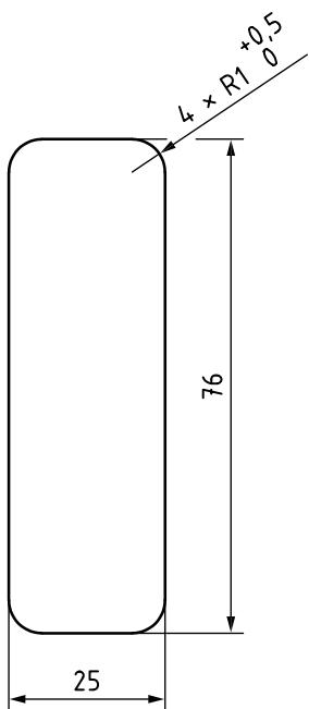
All radii marked shall be 1 mm with a tolerance of 0 mm to +0,5 mm.
