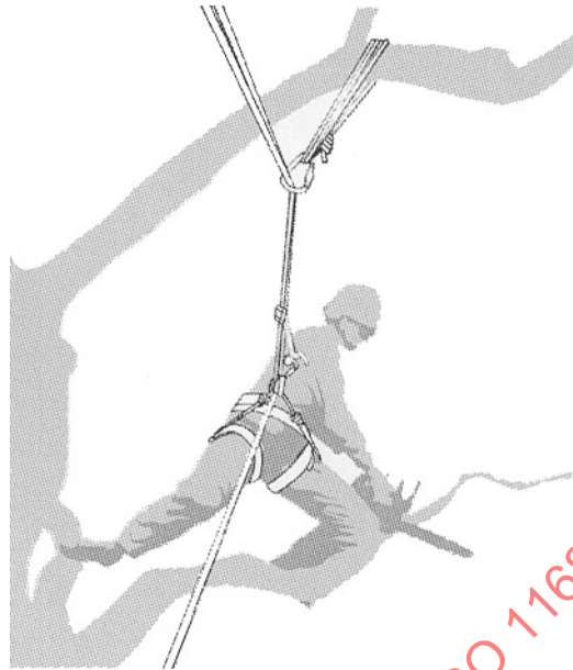
Figure E.3 — Example of redirection of the main line via supplementary anchor point
