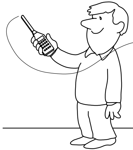
Figure 2 — Example for movement of the sound level meter
