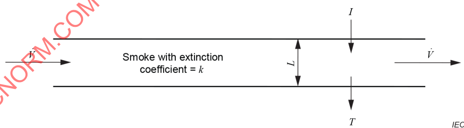
Figure 4 – Dynamic smoke measurement
