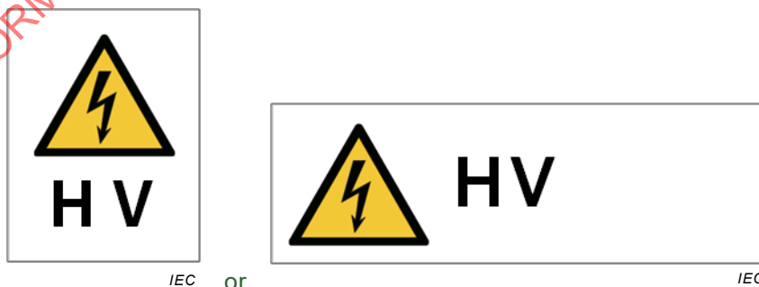
Figure 4 – Warning sign “high voltage”
