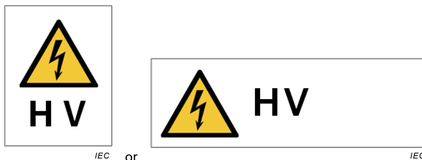
Figure 4 – Warning sign “high voltage”
