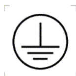
Figure 3 – Symbol for protective earth (protective ground)
